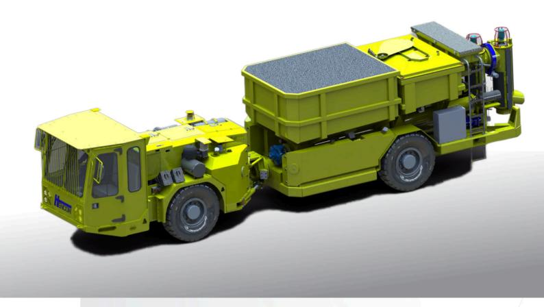
The Hencon TransVers High Profile Batch Mixer has been designed for the preparation of concrete mixtures that are used in Hencon Shotcreter machines.
