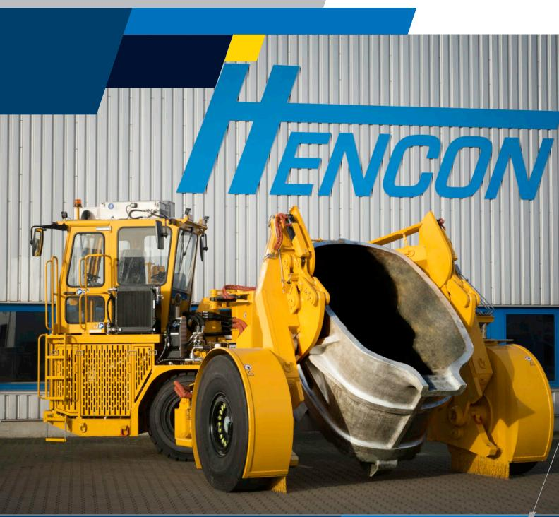
VEHICLE FOR LIFTING, TRANSPORTING AND TILTING OF POTS CONTAINING FERRO-CHROMIUM SLAG
