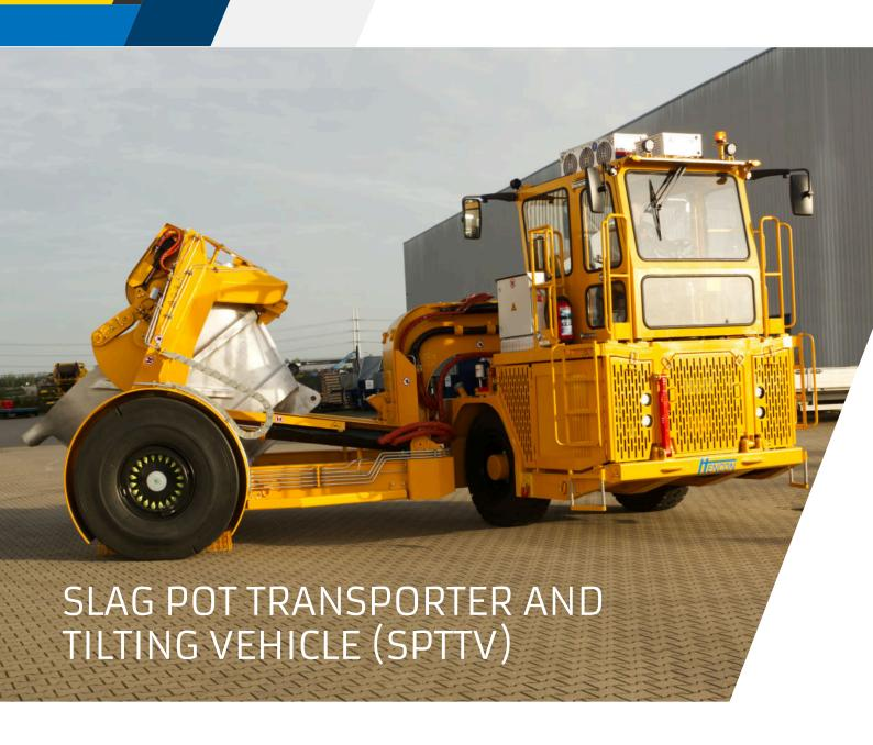
**The Hencon Slag Pot Transporter and Tilting Vehicle** (SPTTV) has been designed with various specialised features enabling it to pick up, transport and tilt pots filled with high temperature (1 750 - 1 850°C) ferrochromium slag or waste matter between furnaces and dumping sites.
