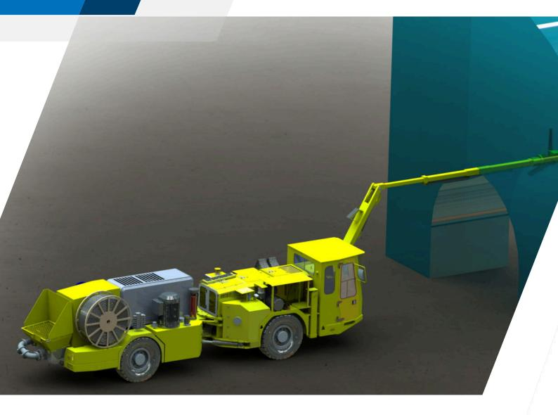
The Hencon High Profile Shotcreter has been designed to spray wet concrete mixture onto the walls of underground tunnels for reinforcement.
