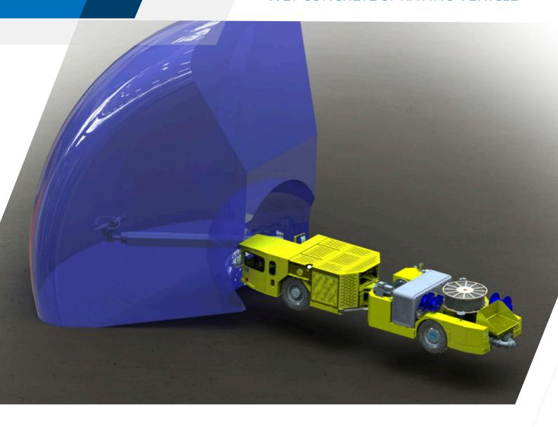
The Hencon Low Profile Shotcreter has been designed to spray wet concrete mixture onto the walls of underground tunnels for reinforcement.
